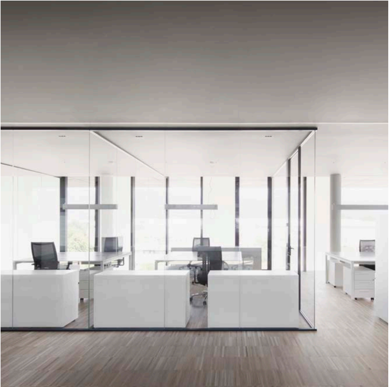
covering: custom bleached oak panel core: calcium sulphate dimensions: 600x600 mm
