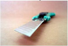
Step 2: Remove the silicone from the sides of the floor panel, use a spatula by inserting it into the edge of silicon. Lever up and remove the silicone from the gap between the two panels. Hold firmly, yet gently pull, the silicone. As you pull, use the spatula or razor blade to loosen the silicone constantly. Work slowly. You can remove more silicone in this way than by pulling and scraping.
